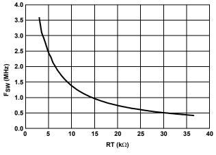
FIGURE 4. FREQUENCY vs RT RESISTOR
