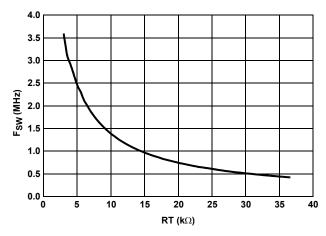
FIGURE 10. FREQUENCY vs RT RESISTOR
