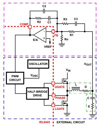
FIGURE 14. VOLTAGE-MODE BUCK CONVERTER COMPENSATION DESIGN
