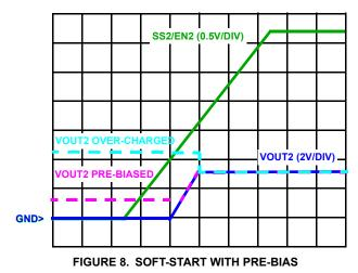
NOTE: Neither output cannot be independently disabled during power-up; both SS/EN pins are pulled low internally during POR, and due to the internal switch, neither will start charging if either pin is still
