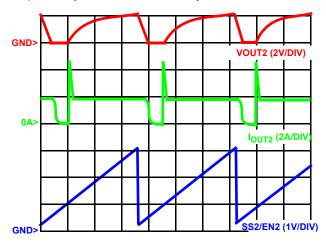
FIGURE 12. OVERCURRENT PROTECTION
